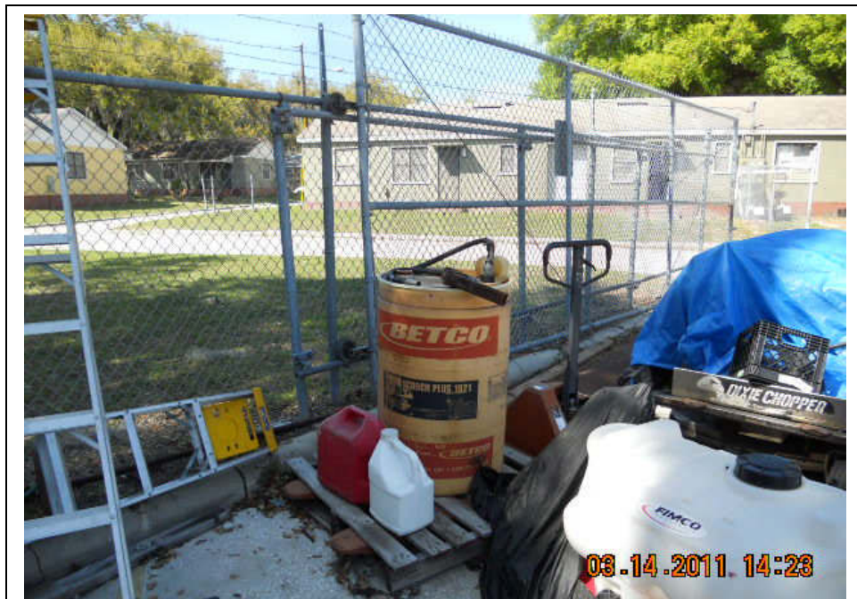
Photograph 16: 55-gallon drum of herbicide stored on wooden pallet atop impervious concrete.
